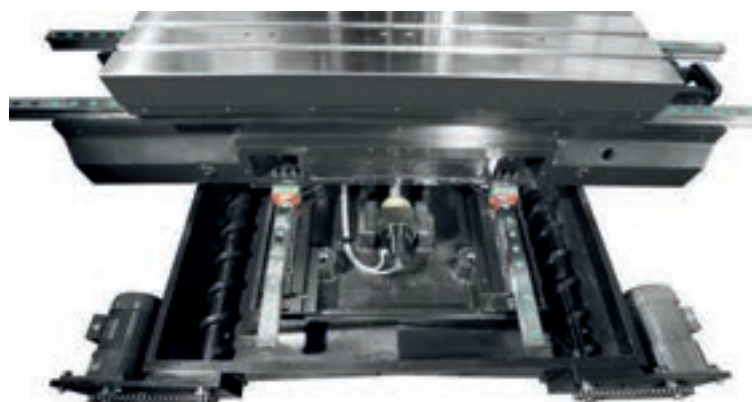
Two screw type chip conveyors in Y-axis (VF1100 & VF1300)
