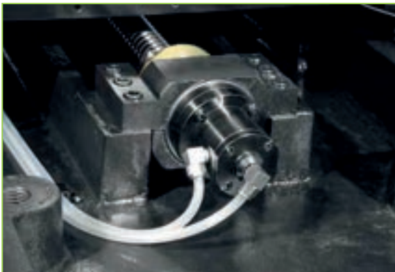
Oil cooling through ballscrew(Only available on VF1100)
